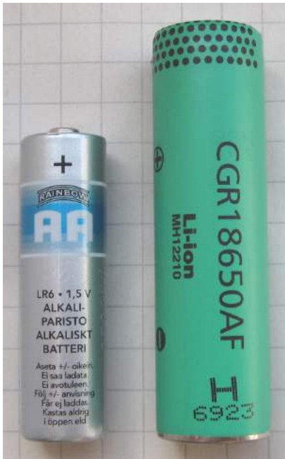
LI 18650 battery – 18 mm in diameter and 65 mm tall
